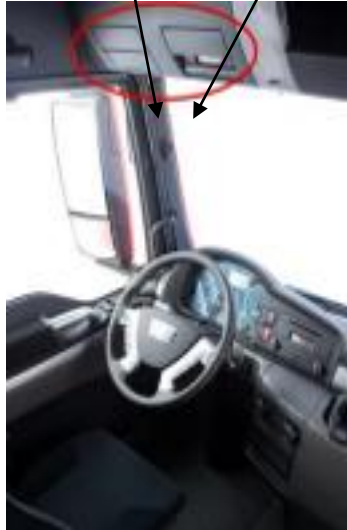
Area to place unit and DTCO harness
